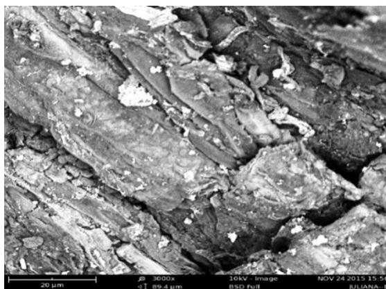
**Plate 2:** SEM Micrographs of unloaded adsorbent (a) and spent adsorbent for Pb<sup>2+</sup> (b)
